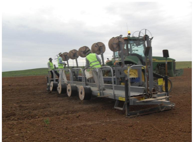
Figure 1: Installing sub-surface drip irrigation
