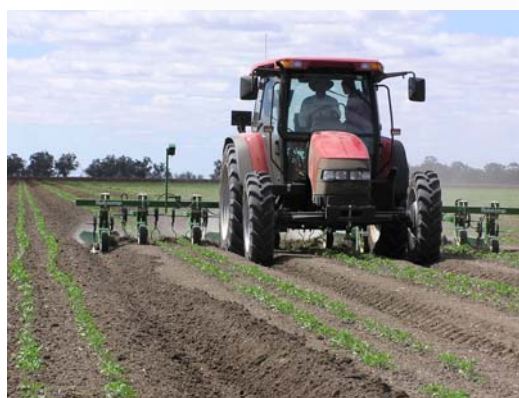
Figure 1: Robocrop precision tillage bar cultivating at 10km/hr in direct seeded processing tomatoes
