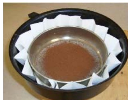
2 - Dry soil sample in sieve over filter
