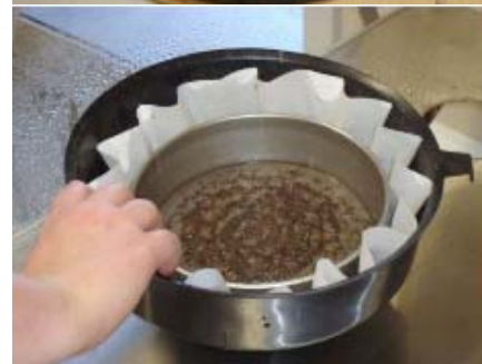
3- Stable aggregates stay in the sieve
